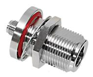
N Female / SMA Female. Connect N plug to SMA plug with GRF05-0021 panel mount adapter. Nickel-plated brass body and hex nut. Gold-plated BeCu contact. Stainless steel lock washer, PTFE insulator, silicone O-ring.
