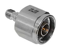
NMale/SMA Female. Connect N jack to SMA plug with GRF05-0019 adapter. Stainless steel body with gold-plated BeCu contact, PTFE insulator, nickel-plated phos bronze lock ring, and silicone gasket.
