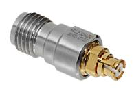
SMP female / SMA Female. 852-175 adapter connects male SMP to male SMA connector. Stainless steel body, gold-plated BeCu contact, PTFE insulator. Gold-plated BeCu anti-rock ring.
