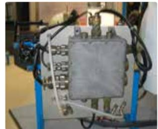
The case was solved with Glenair ITS reverse bayonet connector cables and flange mount receptacles. Plugs with cable clamp backshells mated to receptacles mounted on existing metal junction boxes along with a specially-designed, corrosion-free and EMI/RFI-protected Glenair Composite Junction Box, factory wired to an internal termination block.
