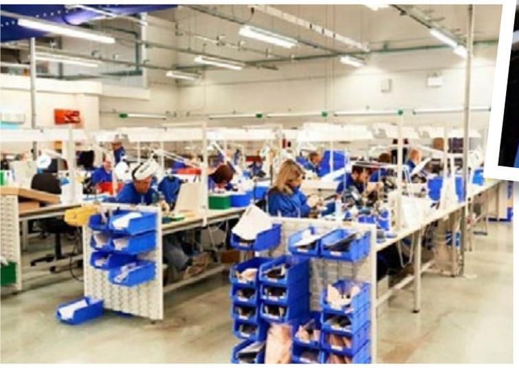
**The Glenair Mansfield clean room assembly area is used for fabrication of laser, space, and satellite assemblies IAW ISO Class 8 -100,000 PPM**
