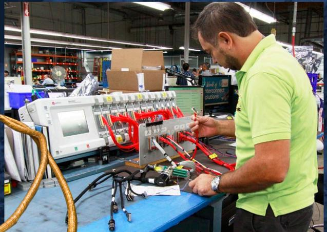
Continuity testing standard on all cable circuits
