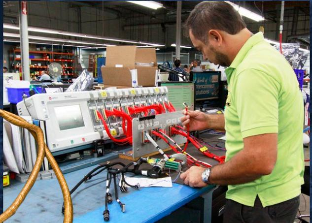
Continuity testing standard on all cable circuits
