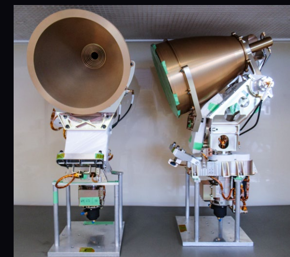
Complex wave guide gain horn assembly with GSS-fabricated components and bespoke shielded wired harness assemblies
