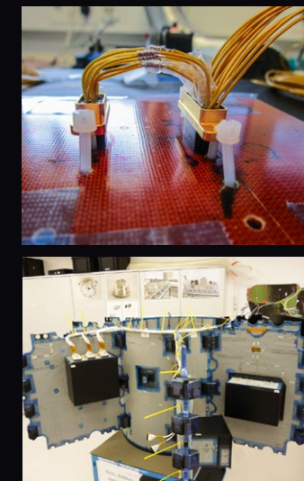
Example of ground support flat set harnessing used in developmental stages of satellite modeling, mockup, test, and mission simulation. Glenair Space Systems manages the entire process, from test cable design and fabrication to mockup integration.
