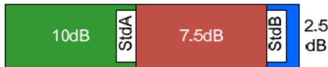
**Figure 1. Original SuperSpeed Gen 1 Loss Budget (from USB 3.1 Channel Loss Budgets).**
