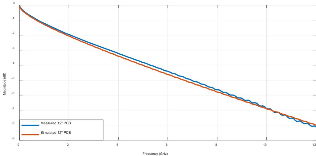
Figure 7 – 12" Link Insertion Losses
