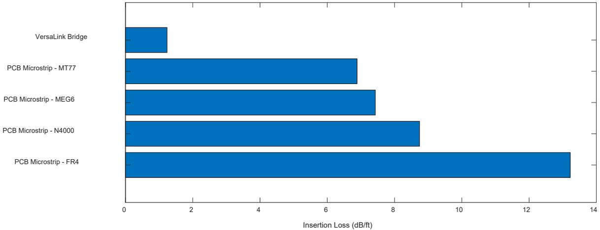
Figure 8 – 12" Link Insertion Loss at 10GHz
