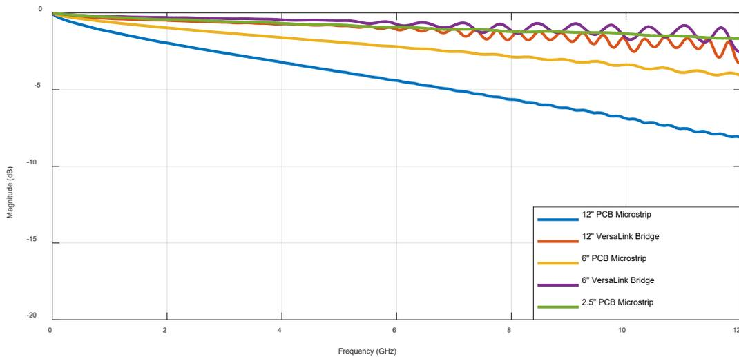
Figure 3 – VersaLink Bridge and PCB Microstrip Insertion Loss
