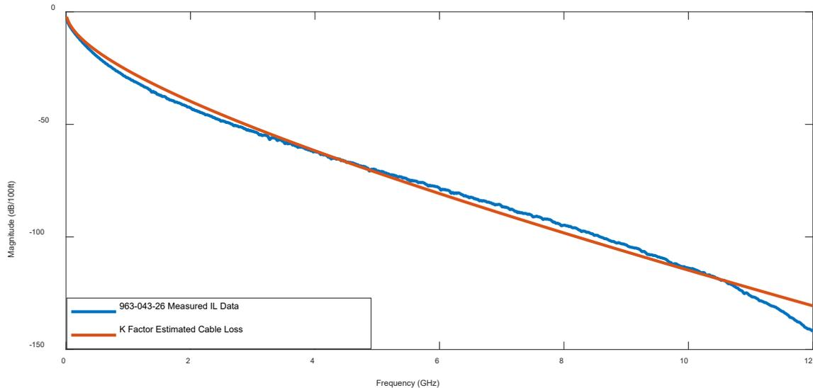
Figure 5 – Measured Cable Loss to Estimate Loss Fit
