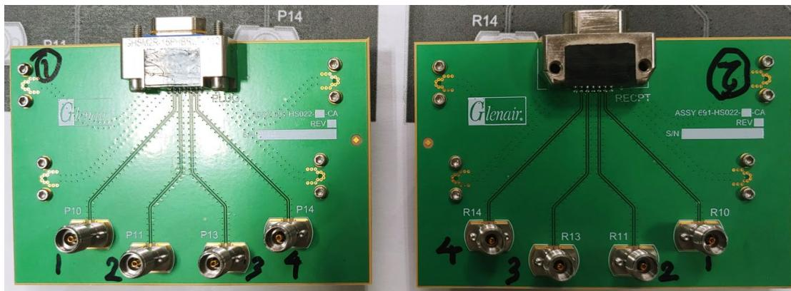
Figure 2. Right-Angle GHSM (HBR) Test PCB Set
