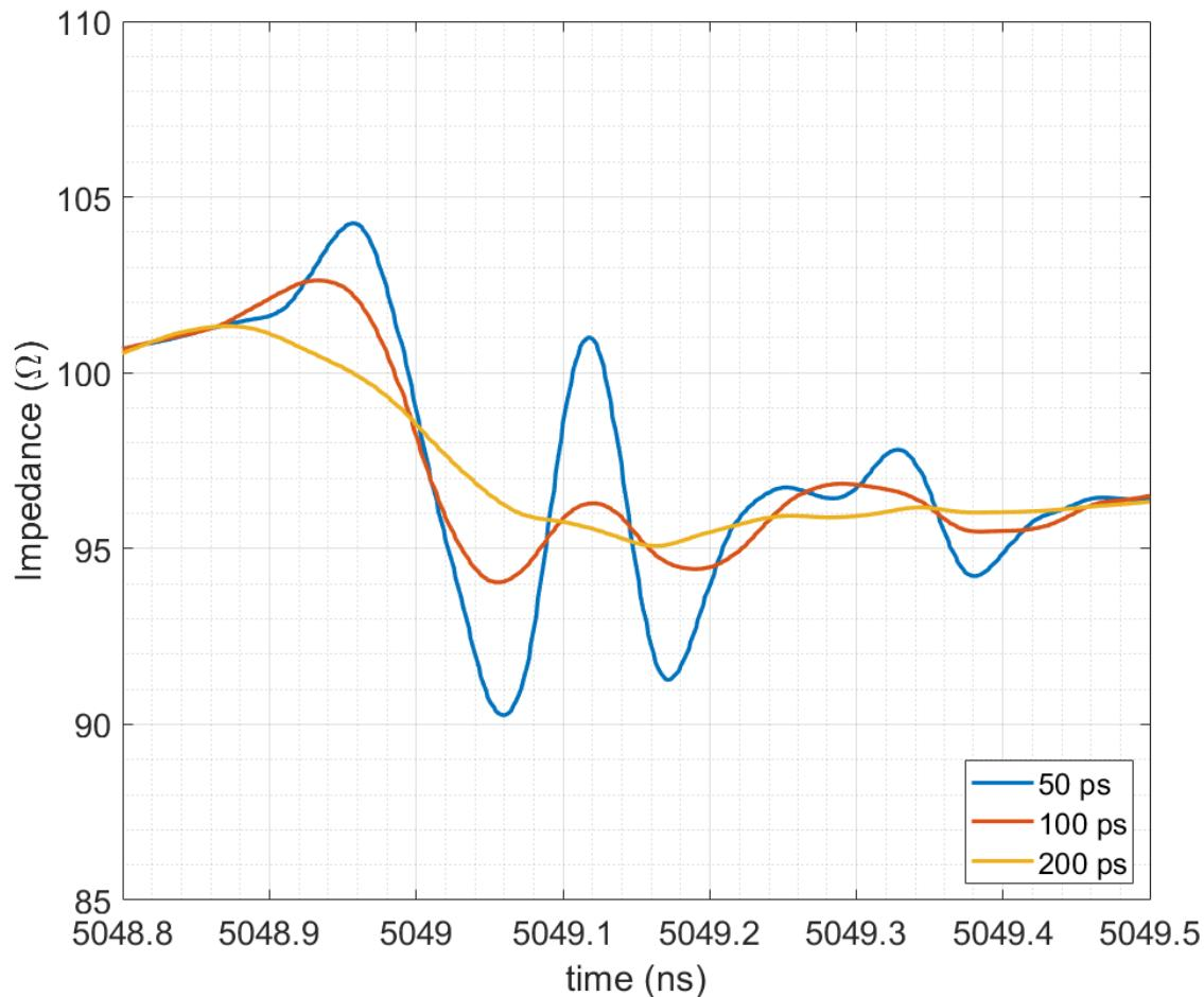
Figure 22. TDR – Straight to Right-Angle GHSM SMT
