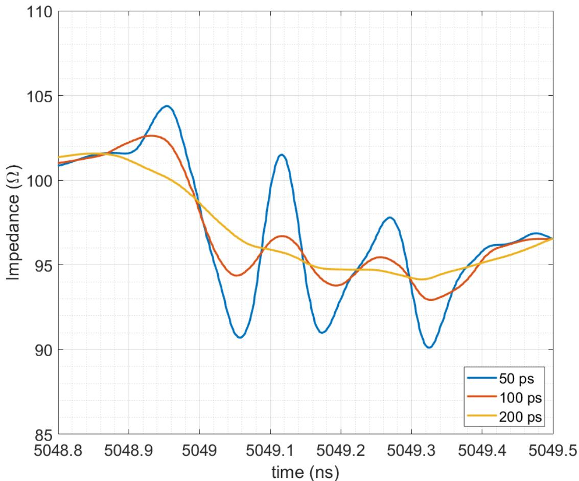
Figure 21. TDR – Straight to Right-Angle GHSM PTH
