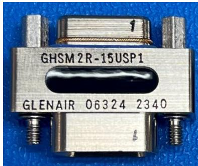
Figure 6. GHSM Sav-Con Connector Saver Test Sample
