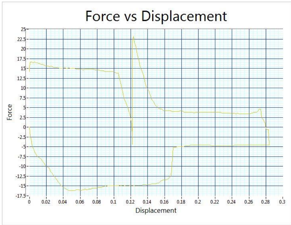
Figure 26: Sample 2B-1B Post Humidity Mating and Unmating Force Trace
