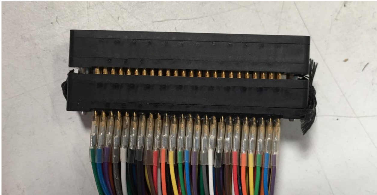
Figure 20: Stacker Test Sample Attached to Adapter for DWV Testing
