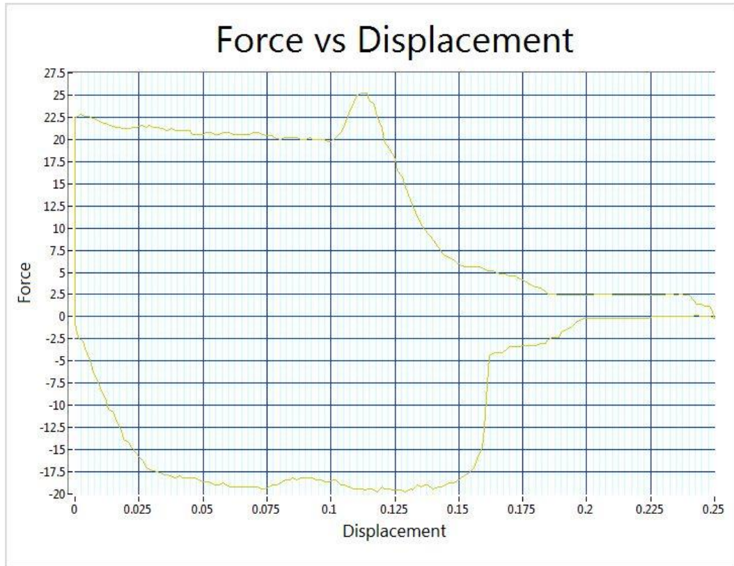
Figure 18: Sample 2A-1A Mating and Unmating Force Post Vibration and Shock
