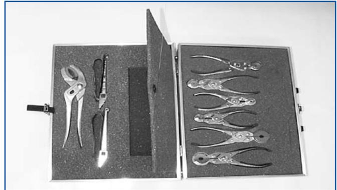
Glenair's TG80 Tool Kit is designed for field use with circular electrical connectors. The products included with this kit fit most connectors covered by Military Specifications, and are used for holding during assembly and disassembly of rear clamp and adapter hardware, and to facilitate connector field repairs and servicing.
