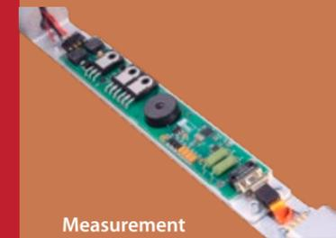
Measurement While Drilling (MWD) tool module
