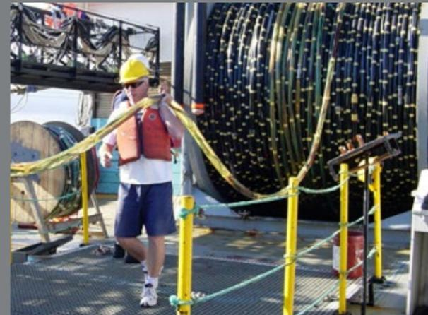
Power and data interconnects for towed-array streamers
