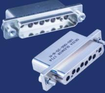
Support from four to twelve GFR termini with insertion loss performance comparable to industry-standard MIL-PRF-29504. Precision-machined with integral alignment pins for optimum optical fiber alignment and low dB data loss performance. Available in aluminum and stainless steel with standard jackpost hardware included. Termini sold separately. Support for single- and dual-O-ring termini. Panel cutouts IAW MIL-DTL-24308.
