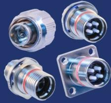
Support from two to twelve GFR pin or socket termini with insertion loss performance comparable to industry-standard MIL-PRF-29504. Precision-machined with O-ring environmental seal. Back-end threads and teeth accept Glenair Mighty Mouse accessories. Available in aluminum and stainless steel. Termini sold separately. Support for single- and dual-O-ring termini.
