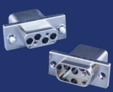
Support from one to eight GFR termini with insertion loss performance comparable to industry-standard MIL-PRF-29504. Precision-machined with integral alignment pins for optimum optical fiber alignment and low dB data loss performance. Available in aluminum and stainless steel. Termini sold separately. Support for singleand dual-O-ring termini. Panel cutouts IAW MIL-DTL-83513.
