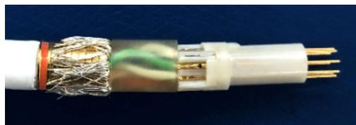
**Inspection Step:** the gap between the plastic bushing and the adjacent component shall be less than 0.010”.
