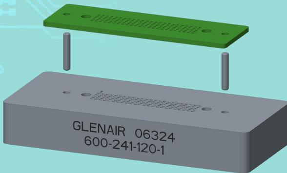
2. Place the board on the support plate and align board clearance holes with the guide pins.
