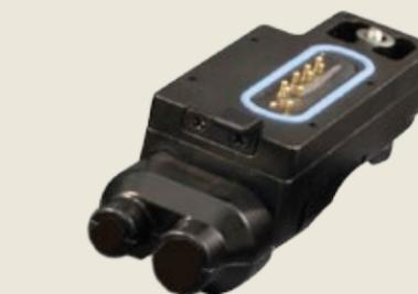
AN/PRC-148, AN/PRC-152, 152A, 154 and RF-7800T Radio Connectors with Series 804 Mighty Mouse Push/Pull Interface. Radio connector cables are available as cabled, un-cabled, and pigtail versions. Radio interface features spring-loaded contacts for reliable and mating and are 100% electrically tested for shorts, continuity and insulation resistance at 200 Megohms minimum.
