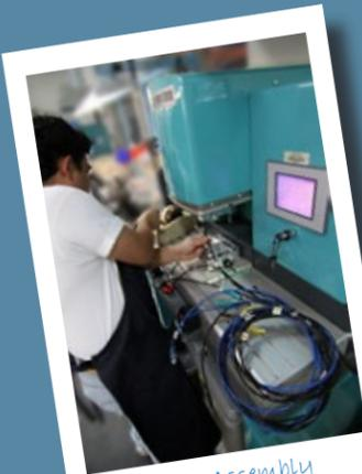
Cable Assembly Overmolding
