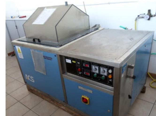
**Accelerated harsh-weather testing** is performed to ensure components under test meet qualification requirements for galvanic corrosion and resistance, resistance to solvents, and SO2.
