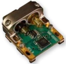
**Advantages of Active Opto-Electronic technology:** leverages the advantages of fiber media, reduces the complexity of fiber optic systems, and excels in harsh application environments.
