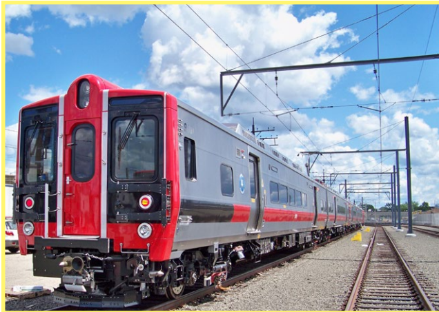
The M8 is an electric multiple unit (EMU) railroad car built by Kawasaki for use on the New Haven Line of the Metro-North Railroad. Photo: office of Dannel Malloy
