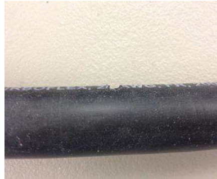
Figure 2: Images of 2/0 Wire After 10,000 Cycles and 0.026 Inches of Penetration
