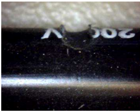
Figure 3: Images of 4 AWG Wire after 30,000 Cycles and 0.043 Inches of Penetration
