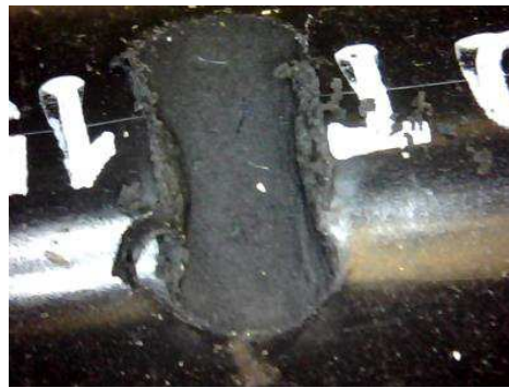
Figure 3: Images of 4 AWG Wire after 30,000 Cycles and 0.043 Inches of Penetration
